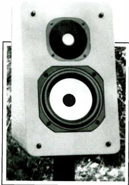
PHOTO 1: Front view of the Sapphire II mounted on the AC Stands. The grille cloths are attractive, but should be removed for the best stereo imaging.
