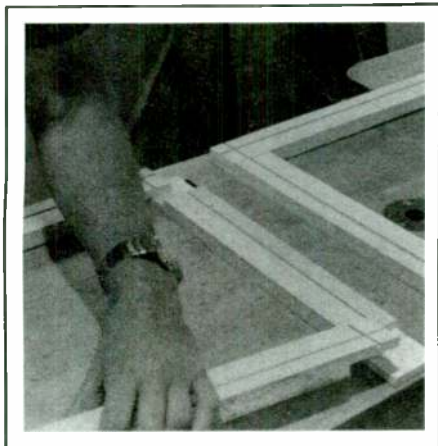
PHOTO 9: The bass grille frame is held with pins and velcro fasteners.
