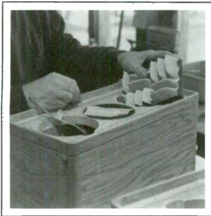
PHOTO 6: Acoustic foam separates the mid-bass drivers.
