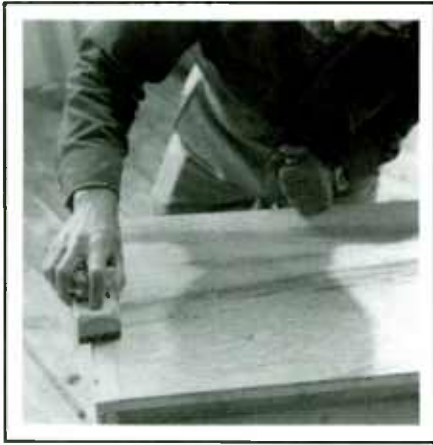
PHOTO 4: Round the corner pieces with a sharp plane.
