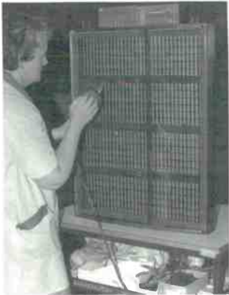
Fig. 14. Joan Lawson uses a heat gun to remove wrinkles from the dust cover of the speaker's diaphragm.
