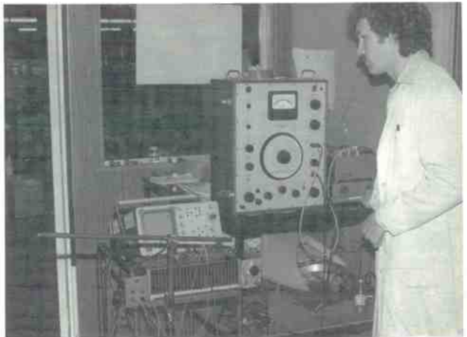
Fig. 17. Richard Ramsey does the "cloning" test where the production line model is tested against a measured standard speaker using a square wave, inverted in one, and both equidistant from a probe mike. A good speaker "cancels" the standard one.
