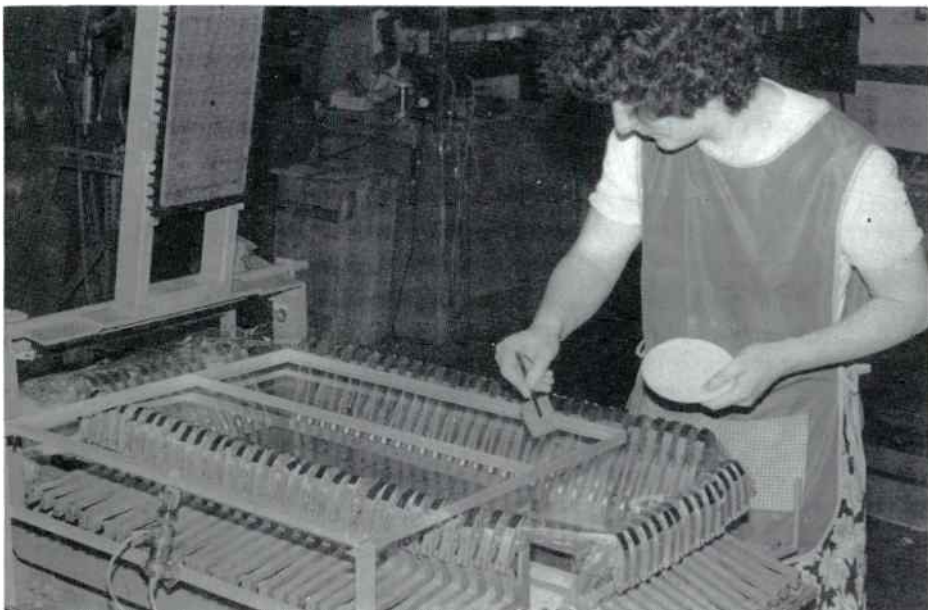
Fig. 11. Lesley Richmond spreads a graphite slurry over the film before bonding it to its frame. The liquid makes the diaphragm slightly magnetic.
