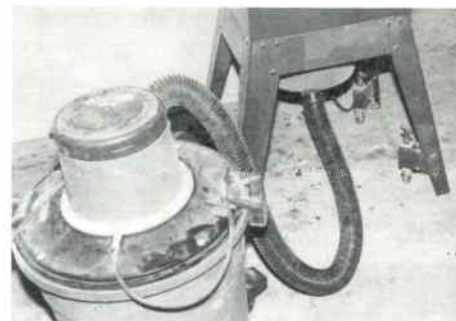
Fig. 8. Vacuum attachment for the table saw.
