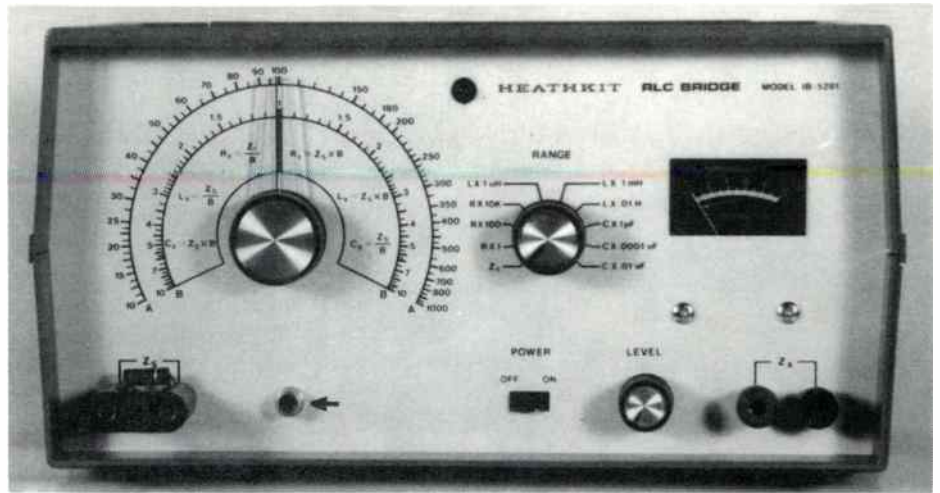
Photo 1. Arrow shows input jack added to front panel.
