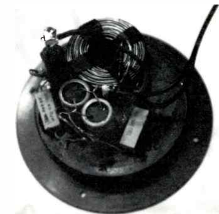
Fig. 6. The base with the crossover components in place.
