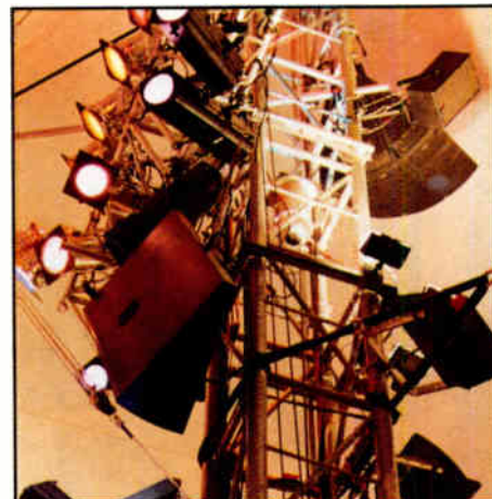
Eighteen Clair Brothers' P-4 loudspeakers were flown in several clusters, as well as individually, on both the four mast poles and a mainframe rigging arch positioned over the stage area.
