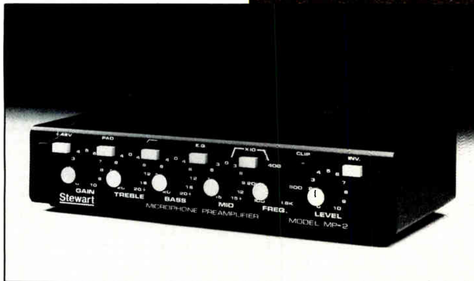
Stewart Electronics' mic/preamp has balanced input/output and EQ settings which can be used as anti-aliasing filters with SYSid.
