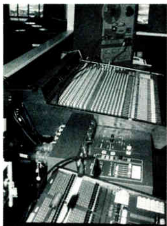
The control booth at the Crystal Harmony's Galaxy show lounge uses a 32-channel TOA mixing board.
