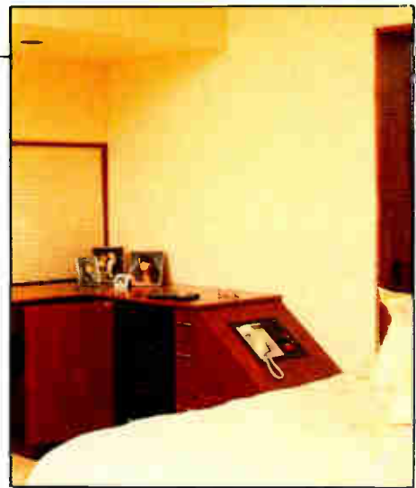
Angled control panel in bedroom contains Yamaha RX-1100 receiver, KXW 900 cassette deck and Echo Star 3000 IRD Satellite tuner.
