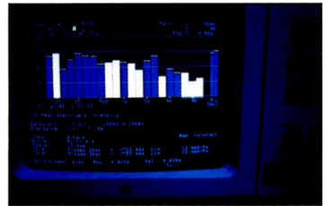
4) At left, polar response showing variation of the measured intensity as a function of angle of incidence for the 4181 in the 3519 probe. 4A) Shown above is a view of the 1/3-octave screen display.
