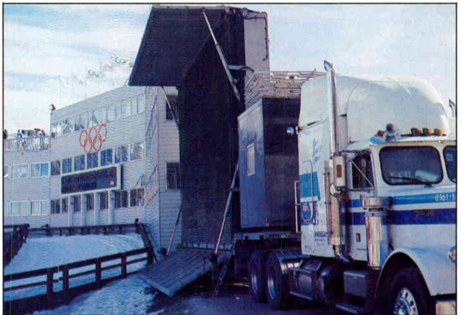
This huge screen called Star Vision, supplied by Avesco Screen Co. of Surrey England, is a matrix of 1,000 CRTs. It was used at the cross country skiing site.
