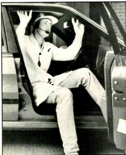
An inspector from Austin-Rover is verbally inputting data to a central computer while performing quality checks.
