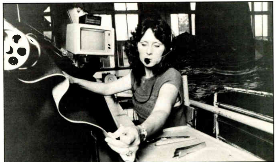
Worker at West Point Pepperell's textile plant puts information into a computer by speaking into Votan equipment.
