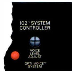
Rear panel control for voice-channel gain.
