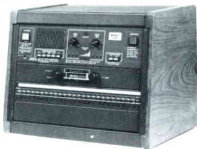
The Ring 3000 School System, a two-channel system, can service up to 500 different rooms providing selective and all-call announcements, program feed and other features.
