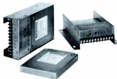
MacKenzie’s new, solid-state Digital Message Repeaters use EPROM memory cartridges to play messages. The sound is excellent—and completely natural.
