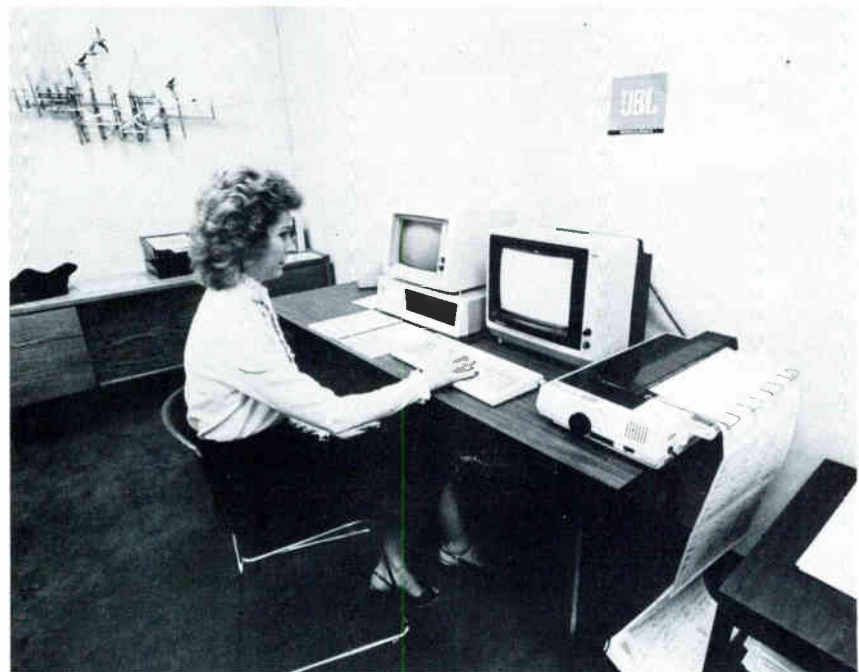
Francie Wuilley of JBL at the console of the IBM Personal Computer. The main display screen is in the center, the magnetic disc unit is on the far left, on the bottom, and the dot-matrix printer is on the far right of the table.
