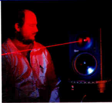
Mackie acoustic engineer David Bie uses scanning laser vibrometry to map HR824 tweeter dome vibrations. Film at 11.
