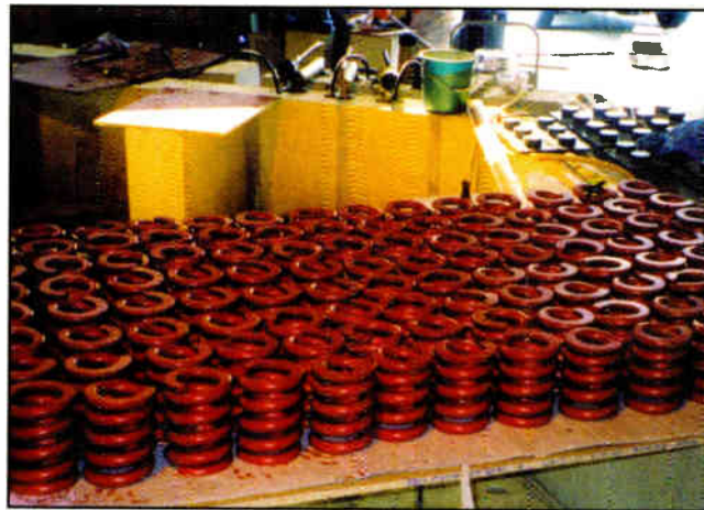
Helical springs are placed under the floor slabs of all of the studios and the control room.
