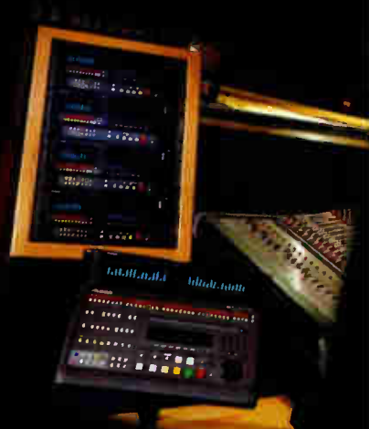
32-track M20 system with CADI™ Remote/Autolocator and RMD™ Meter Display at The Village, Studio D, West Los Angeles, CA
