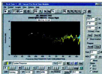
Figure 3: The transfer function display shows frequency response in the familiar dB vs. frequency format.
