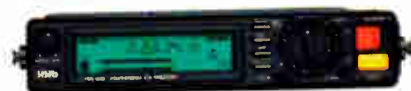
PDR1000 4 head, 4 motor portable professional DAT recorder with 44.1/48/32kHz recorder, balanced XLR analogue I/O and AES/EBU + SPDIF digital I/Os.
