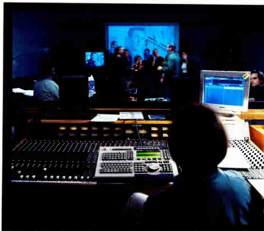
ADR assistant Steve Fitzmaurice, far left, sits on Stage 5 with the SuperLoopers while Stacey Michaels mixes at the Trident Series 65. ADR is recorded directly into the Fairlight.
