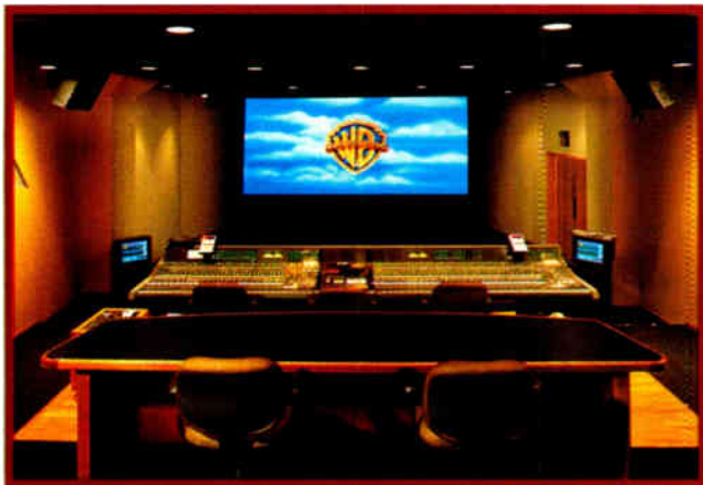
Left: Warner Bros. installed two AMS Neve Digital Film Consoles for use on the long-form TV re-recording stages in Burbank. Each is designed for two-mixer operation and provides 88 inputs, with 72 faders on the surface.
