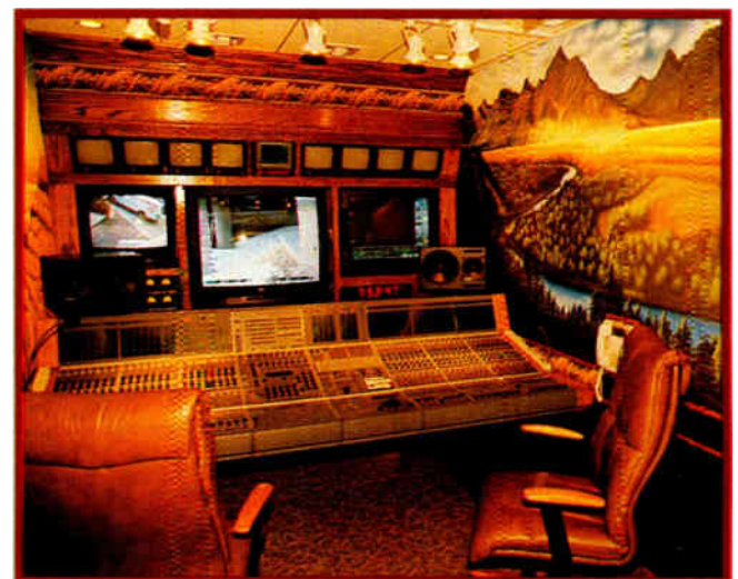
Below: The Nashville Network outfitted its first audio remote truck, equipped with a 48-channel AMS Neve Capricorn. The truck will be used to record live concerts and, when not on the road, will double as a remixing/production station.
