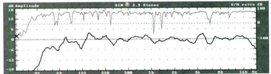
Chart 2: Response of speaker positioned vertically on stand eight inches behind console
