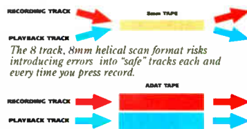
The ADAT format records each track discretely, as all professional multitrack recorders should.
