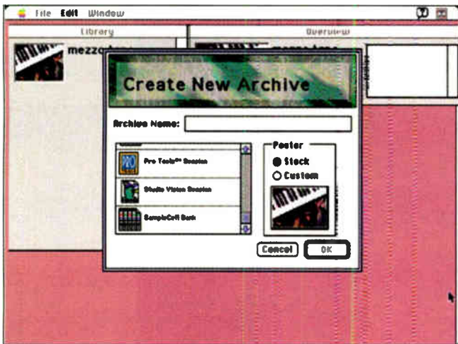
Figure 2: Mezzo archiving software lets you select ProTools sessions, StudioVision files and SampleCell banks, as well as standard Mac data files.
