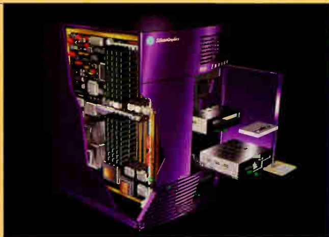
Exploded view of IRIS Indigo workstation.
