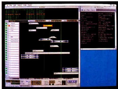
ProDisk's new Graphical User Interface for Digital Editing (guide™) combines several windows into an intuitive, easy-to-use display. Far from just an EDL list, the relationship between all tracks is shown.
