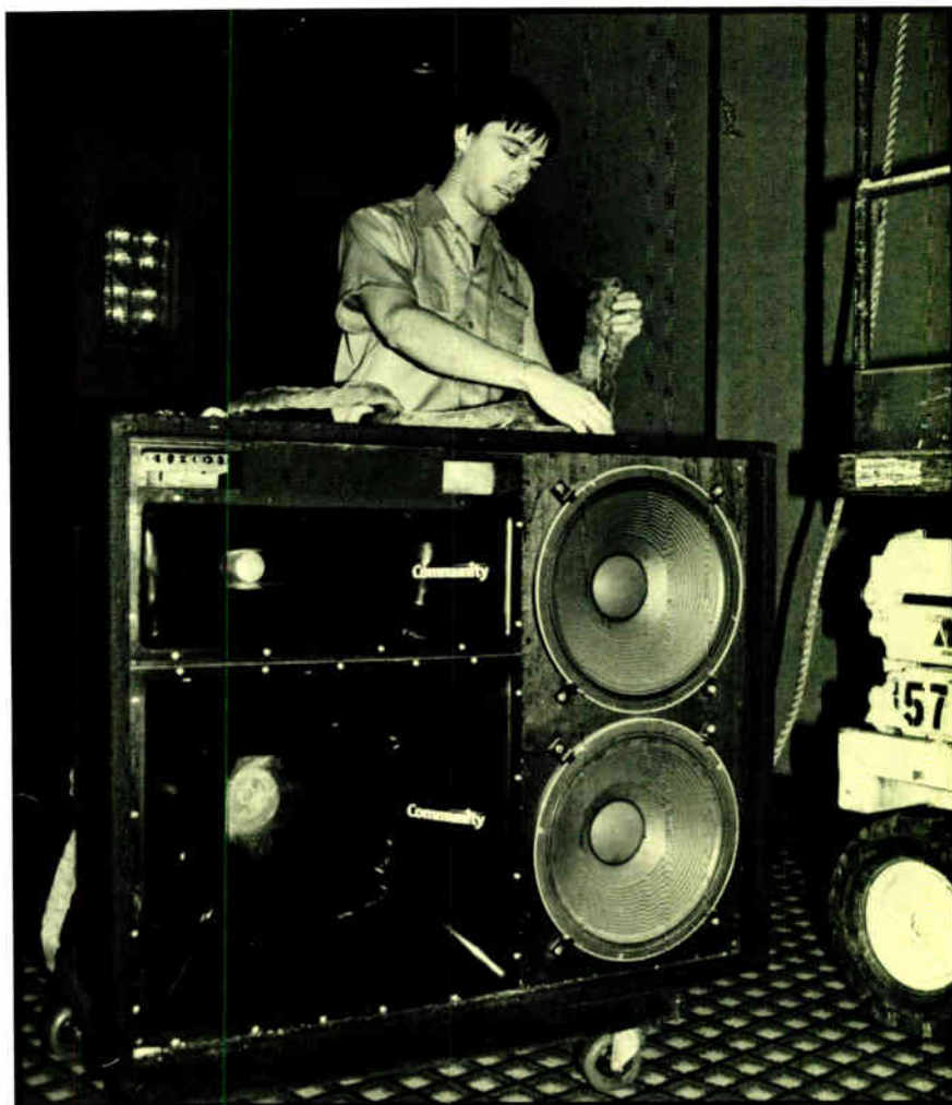
Custom-built for Bally's, these innovative cabinets are designed around Community Light & Sound's mid-range compression drivers.
