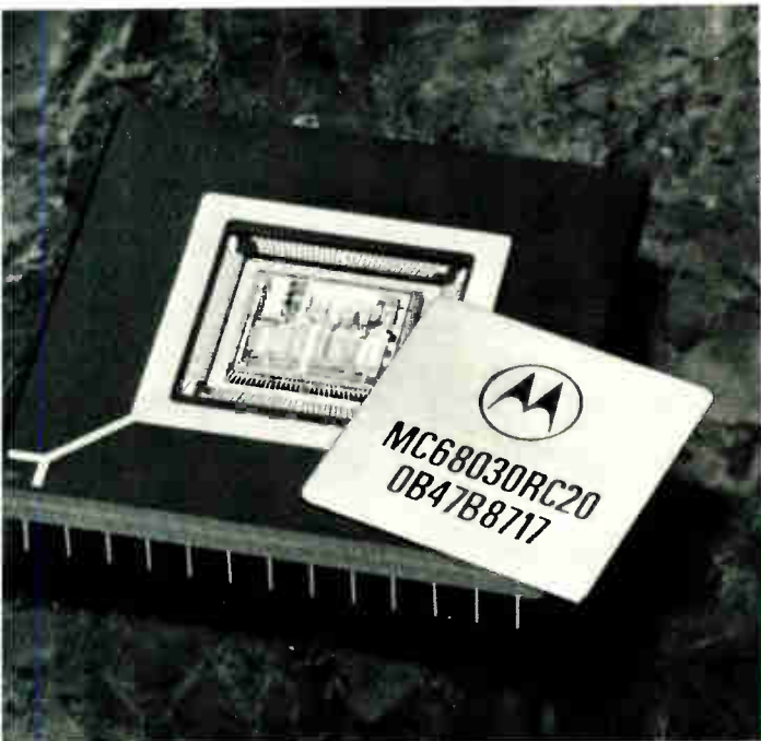
Motorola's 68030 CPU chip has fostered the development of a new generation of powerful workstations.
