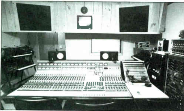
Pictured here is Unique Recording's new "MIDI City" room featuring a 32-channel Neve 8068 Mk II, UREI 813s and a slew of outboard gear. It's adjacent to a small acoustic recording area (through glass) perfect for vocals, percussion, guitar and the like. The room was designed by the Manhattan studio's own Bobby and Joanne Nathan, with acoustical consultation by Bruce Freeman, and equipment supplied by Martin Audio/Video, Manny's Music, Sam Ash Music and Audiotechniques, all NYC businesses.
