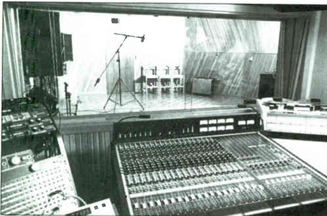
Pictured here is Unique Recording's new "MIDI City" room featuring a 32-channel Neve 8068 Mk II, UREI 813s and a slew of outboard gear. It's adjacent to a small acoustic recording area (through glass) perfect for vocals, percussion, guitar and the like. The room was designed by the Manhattan studio's own Bobby and Joanne Nathan, with acoustical consultation by Bruce Freeman, and equipment supplied by Martin Audio/Video, Manny's Music, Sam Ash Music and Audiotechniques, all NYC businesses.
