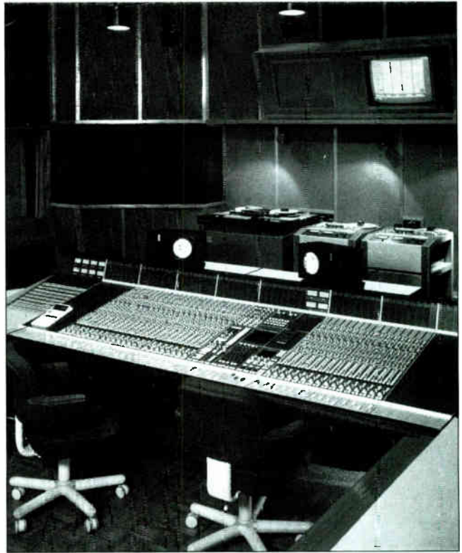
Ardent Recordings of Memphis is the largest studio in Tennessee, and with the addition of Studio B, it's easily one of the best equipped, too. Studio B boasts an SSL 6000E, a Mitsubishi X-850 32-track recorder, and a massive complement of outboard gear.
