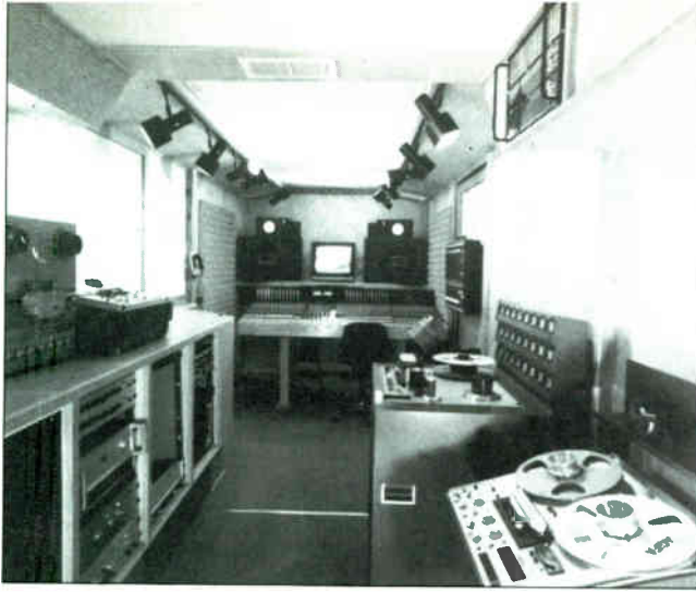
The Big Mo Recording Truck, based in Wheaton, MD, was designed by Ed Casey of Entertainment Sound Production (Washington D.C.) and features a custom 40-input console specifically laid out for remote applications, a Soundcraft sub mixer, two MCI 24-tracks, UREI and Yamaha monitors and a flexible assortment of outboard gear. The control room was built by Bill Hill and Ed Eastridge of Pro Audio, Inc. in Wheaton.
