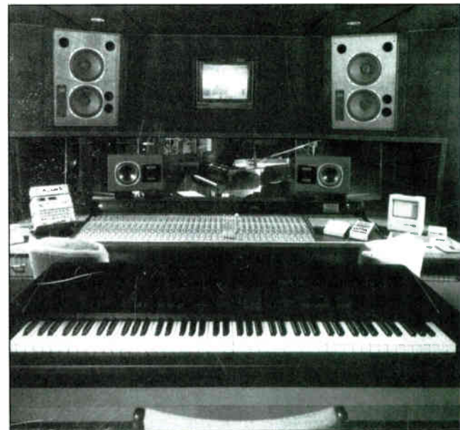
Formerly known as Arthur Smith Studios, Studioeast in Charlotte, North Carolina was completely redesigned this past January by Steve Durr. Supplied by Showcase Audio in Atlanta, Durr installed an Amek Angela 36 x 24 with a pair of Tannoy FSM monitors in conjunction with a Studer A-80.
