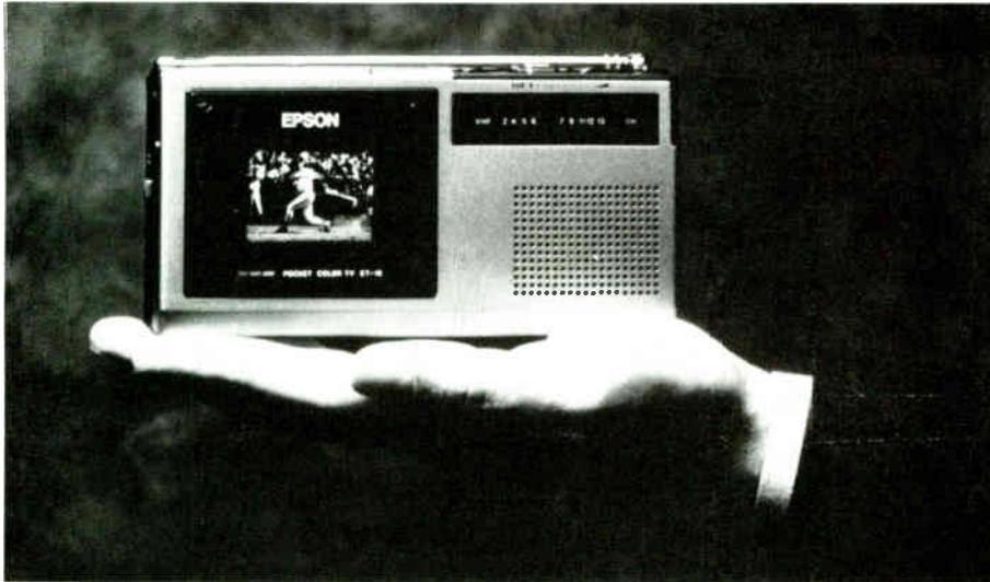
The Epson Elf, the world's first flat screen LCD television, weighs in at just over one pound and has a two-inch diagonal screen.
