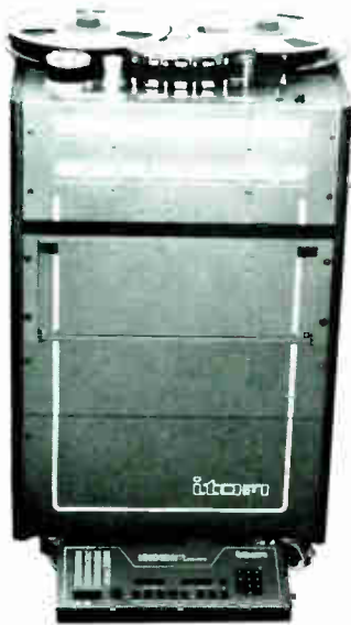
*ITAM model 1610 1"-16 track, 7½, 15 & 30 ips, + 4 in/out, full function remote standard.
