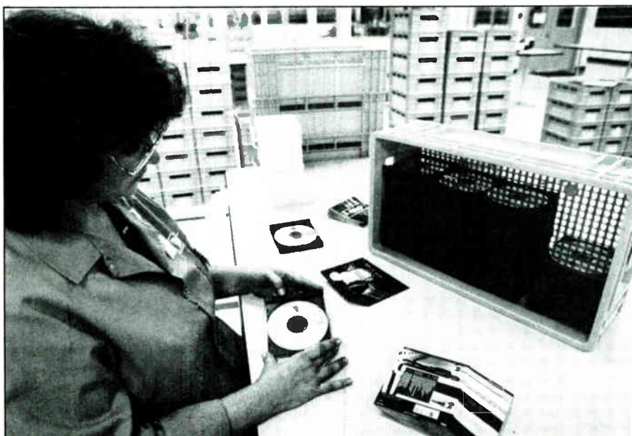
(Below) Stacked on spindles, finished CDs are placed into individual trays which are then packed into clear cases.
