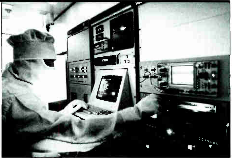
Sony's Compact Disc Master Code Cutter produces a glass master by exposing a glass plate with a photo-resistant layer to a laser beam.
