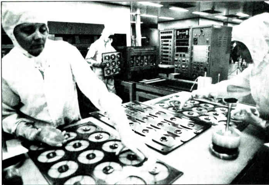
(Above) After injection, a very thin layer of aluminum is placed over the disk's pitted surface that reflects the CD player's laser.
