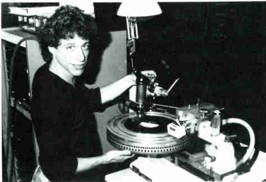
Joe Gastwirt at custom console and lathe which features a JVC quartz-lock motor and proprietary JVC cutter head. The JVC cutting system features 800W/channel threshold amps—JVC Cutting Center.
