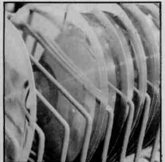
Stampers waiting for centering and processing for press.
