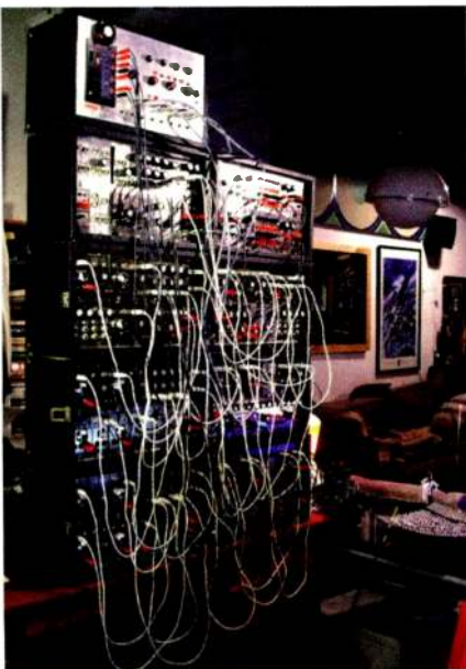
A stack of PAiA 4700 synthesizer modules, wired up and ready to go
