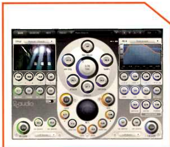
Aether's well-organized GUI offers deep and completely independent control over early and late reflections.
