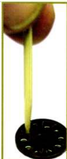
A toothpick or bamboo skewer is handy for cleaning tube sockets.
