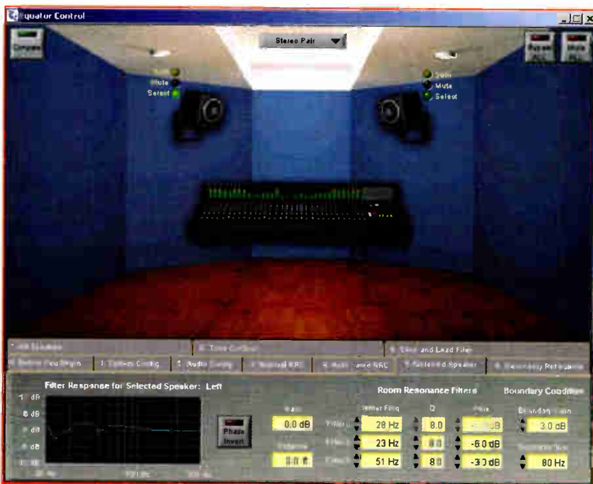
The Equator Control software calculates primary room modes and then instructs the monitors how to correct for room anomalies.
