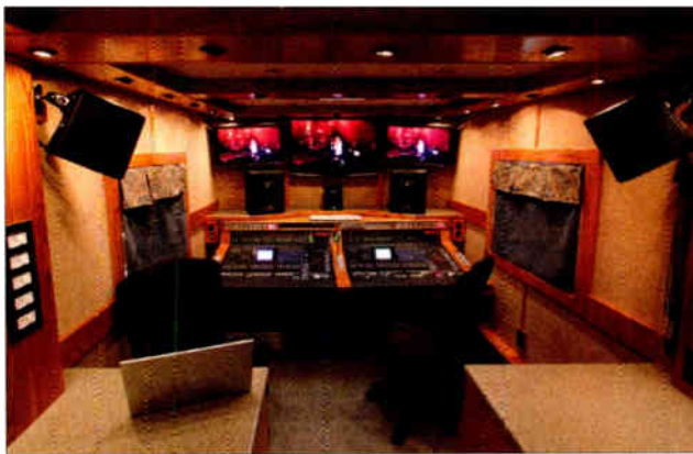
Record Plant Remote's interior: Yamaha DM2000 consoles with fiber optics
