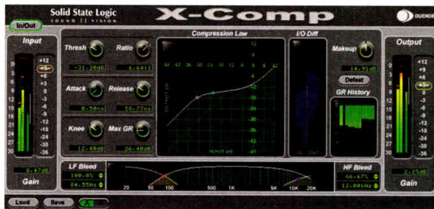
The X-Comp's dual-symmetrical knee design allows detailed shaping of the compression characteristic.
