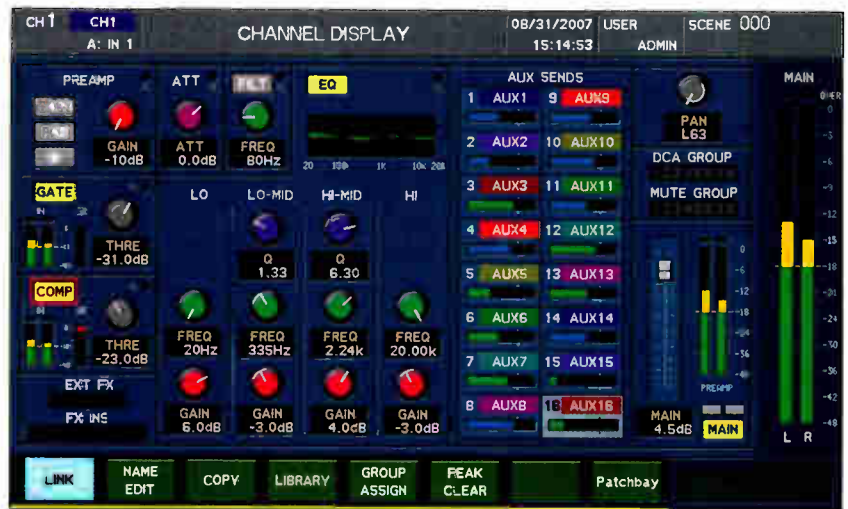
The M-400's Channel Editing display offers an analog-style layout of channel parameters. You can change values using the M-400's dedicated knobs and buttons.
