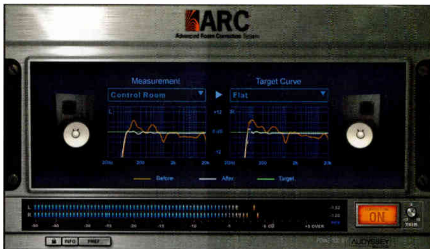
Powered by Audyssey's MultEQ, ARC System's corrective plug-in offers four target response curves.
