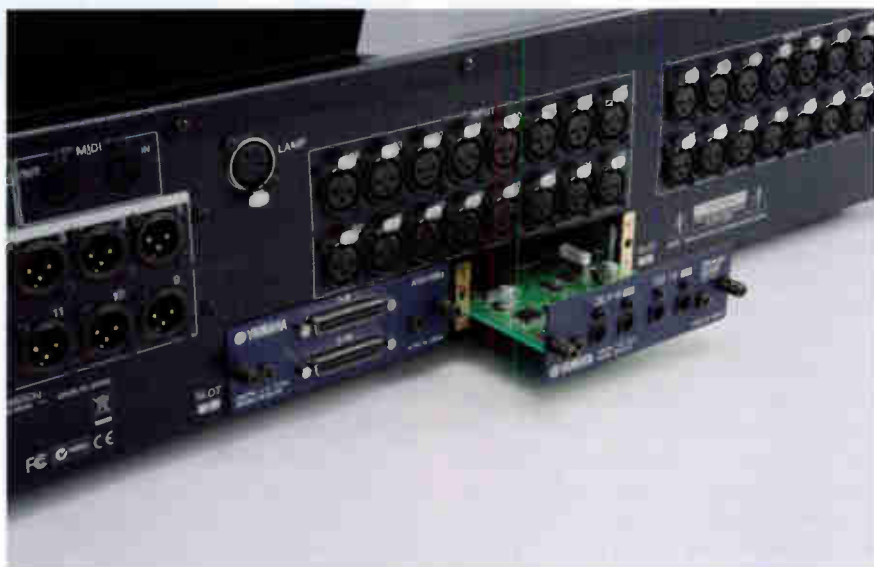
The expansion slot offers TDIF, ADAT, AES/EBU, CobraNet and analog options.
