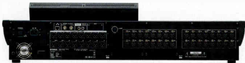
Yamaha LS-9 rear view features XLR I/O, word clock I/O, Ethernet and more.
