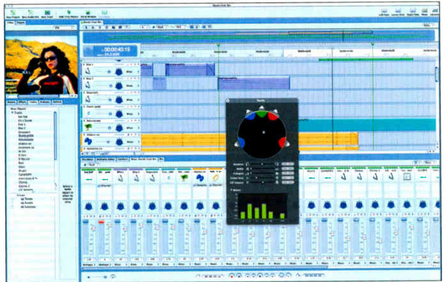
Clicking on a track's surround pan icon brings up a surround panning puck with easy access to parameters.
