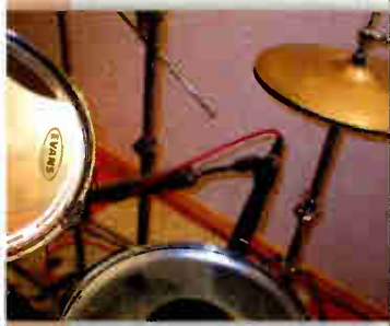
Figure 2: proper position for a cardioid mic on a snare
