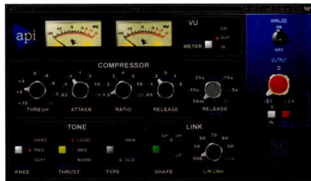
The API 2500 stereo compressor plug-in has separate threshold, attack, release and ratio controls.
