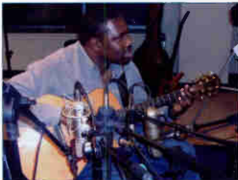
Acoustic guitar miked with RCA 77, Royer R-121, Octavia MC 012, AKG C 414, Neumann KM 184 and U87, and Sennheiser e914
