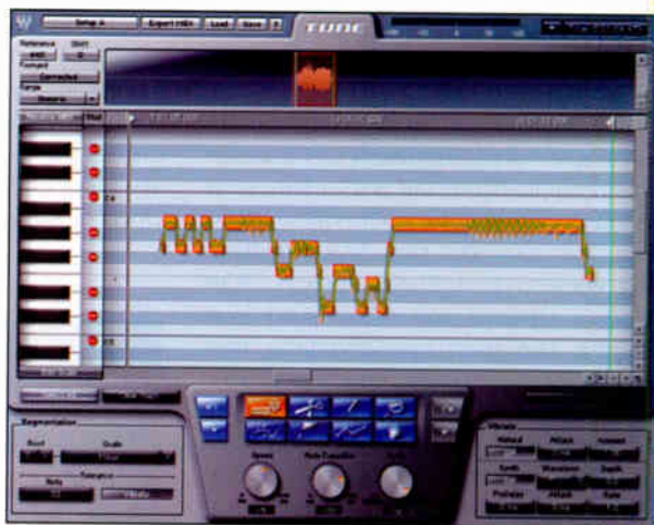
Waves Tune's Edit window shows pitch blocks, and original and corrected pitch.
