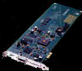
Symphony PCI Card 32 Channels of I/O per card & up to 96 channels per system
