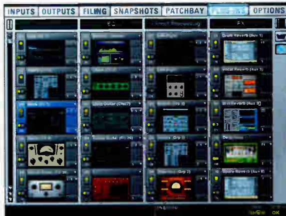
The Plug-Ins tab in the D-Show software can organize up to 100 plug-ins in four user-definable "racks" for fast access.
