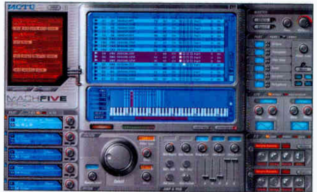
The top-most blue-shaded List Editor screen shows the three lowest-velocity zones (highlighted here) for the same snare drum. Below those in the list, the highest-velocity zone for the same snare is shown to be routed to Insert B. Although Insert effects A and B use the same Simple Reverb algorithm, Insert B's effect is programmed for a longer decay time.
