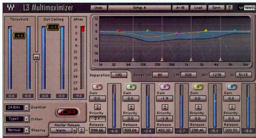
The L3 Multimaximizer interface includes controls for per-band gain, release time and priority.
