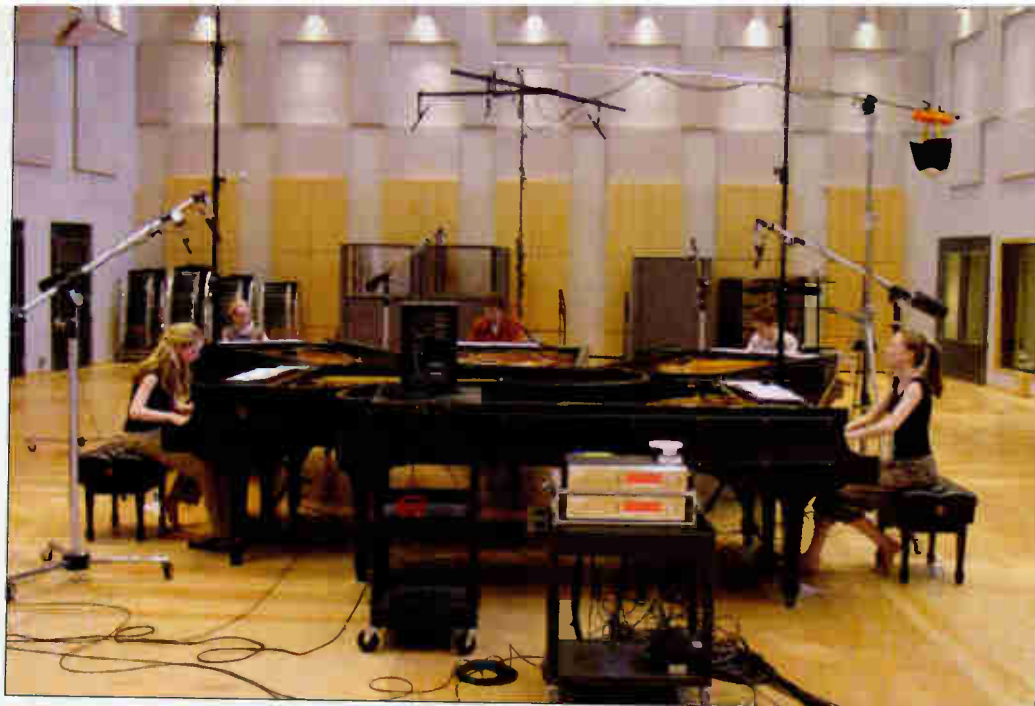
Tracking at Right Track Studios involved a Decca Tree setup of B&K 4006s poised over the 5 Browns' five Steinway pianos.
