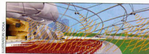
Figure 1: The concentric arrangement of loudspeakers and use of digital delays creates the impression that sound is arriving from the stage.
