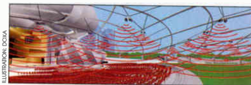
Figure 2: Downward-facing loudspeakers deliver sound that is enhanced by specialized LARES electronics to simulate sound reflections. Laterally arriving sound also masks city noises.
