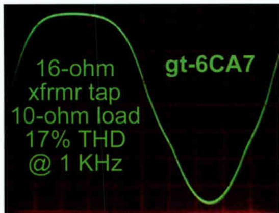
Figure 1b: The Groove Tubes 6CA7, same amp as Fig. 1a, but with the output impedance switch set to 16 ohms and the level adjusted for 17-percent THD
