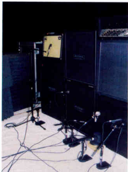
A Mesa Boogie-dominated wall of guitar cabinets fills Tremonti's makeshift amp recording room. An AKG 414, Audix D6, BLUE Dragonfly, Cole 4038 and several Shure SM57s capture the sounds of this mighty rig.
