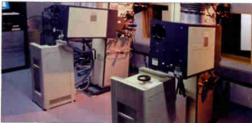
At NT Audio, its projectors (pictured) have five sound heads instead of the normal two.
