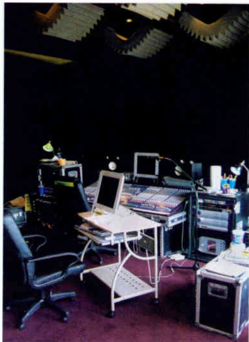
While recording at Tremonti's home, Alter Bridge used the second floor's largest space as a temporary control room. The Pro Tools|HD recording rig used a mostly Neve 1073 front end with a Midas live console.
