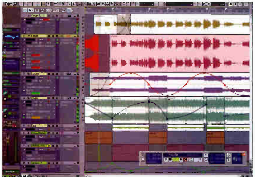
Sonar's Track view displays an overview of track parameters alongside the Arrange window, allowing fast modification without scrolling through the Mixer window.
