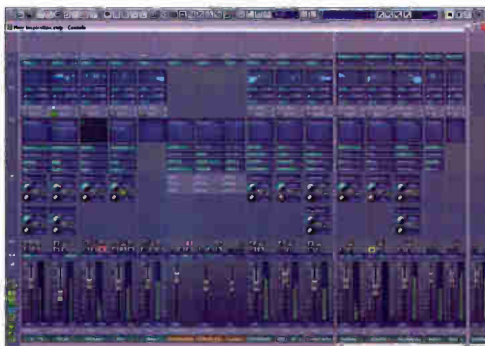
Sonar's Console view can be configured to display or hide functions on a per-channel basis and allows dragging and dropping of effects plug-ins between channels and buses.
