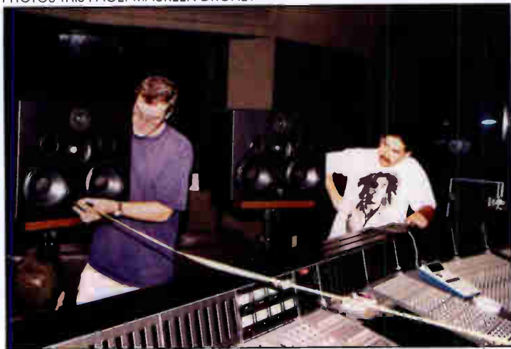
Setting up the mains: Botnick's Quested monitoring system included LCR speakers set roughly in place, tested with pink noise and then fine-tuned with a tape measure and a LaserMark LaserCross. Subwoofer placement is determined by a combination of SPL measurement, Botnick's ears and room logistics. "The best place is near the door," says Botnick with a laugh, "but then someone might trip over it!"
