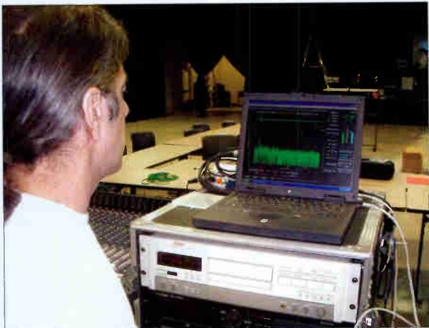
Conservatory instructor Keith Marris uses SIA Smart Live software on a laptop to tune the system and put the quad setup in place.
