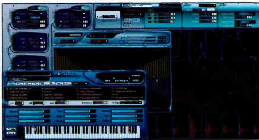
Absynth features a combination of multiple synthesis techniques, with granular sampling and flexible envelope control. Its semi-modular architecture includes more than 800 presets, high-quality filters and LFOs for modulation of parameters.
