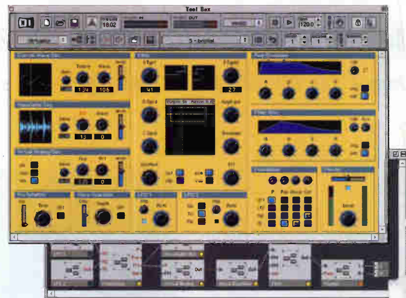
Reaktor features a library of modules, including oscillators, filters, envelopes, LFOs and other mathematical operators. These building blocks let users create their own software synthesizers, samplers, drum machines or signal processors from scratch.
