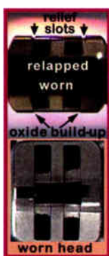
Figure 4: Multiple views showing the effects of wear on a tape head
