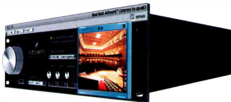
A virtual sampling reverb: The Altiverb plug-in lets you sample your environment and save the set of impulse responses as a preset. You can even import a picture for the scrapbook.
