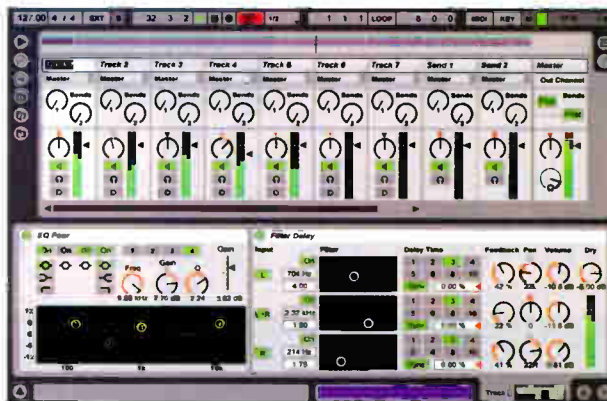
Here are Live's EQ (a 4-frequency parametric EQ) and the impressive, even outlandish, Filter Delay routed pre-fader on Track 1.
