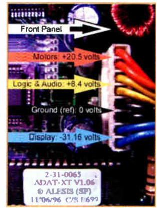
Figure 2: Measuring the ADAT-XT power supply from the main board connector, with the top cover removed.
