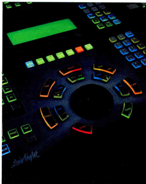
D.R.E.A.M.'s Binnacle editing offers a new approach to workstation ergonomics by centralizing editing and transport functions around a jog wheel, for one- or two-handed editing.
